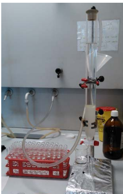
Figure SM 4.1.1.9.5 – Column chromatography performed under external pressure applied by compressed N 2 .
