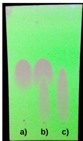
Figure SM 4.1.1.1.4. TLC plate. 60% diethyl ether/petroleum ether. a) cinnamic acid b) cinnamic acid and product c) Product
