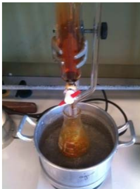
Fig. SM 4.1.1.2.2. Preparation of the perbromide
