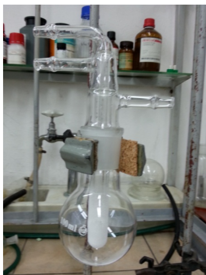
Figure SM 4.1.1.10.8 – An apparatus for the sublimation of isopinocampheol under reduced pressure.
