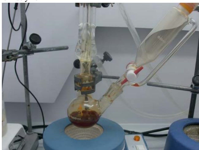
Figure SM 4.1.1.1.3. Reaction apparatus after the Br 2 addition.
