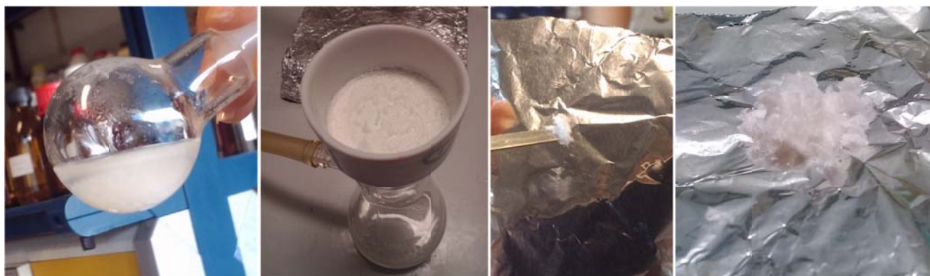
Figure SM 4.1.1.9.8 – Recrystallization of dodecyl 2-deoxy- \alpha -D-arabino-hexopyranoside ( 5 ), from ethyl acetate/ n -hexane.
