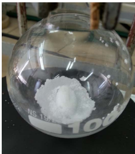
Figure SM 4.1.1.10.5 – Solid d\text{Ipc}_2\text{BH} after washing with hexane. This compound forms large hard crystals.
