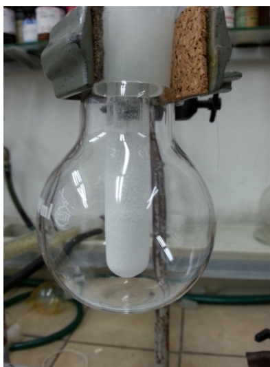
Figure SM 4.1.1.10.9 – Pure isopinocampheol collected on cooling finger after sublimation.
