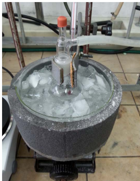
Figure SM 4.1.1.10.4 – Crystallization of d\text{Ipc}_2\text{BH} in water/ice/salt bath (Method 2).
