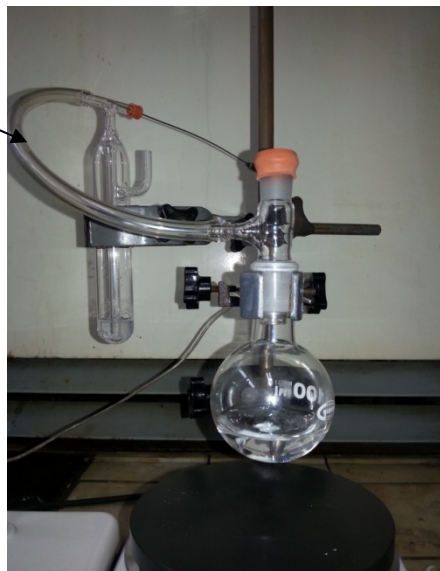
Figure SM 4.1.1.10.1 – An apparatus for hydroboration conducted under an inert gas atmosphere
