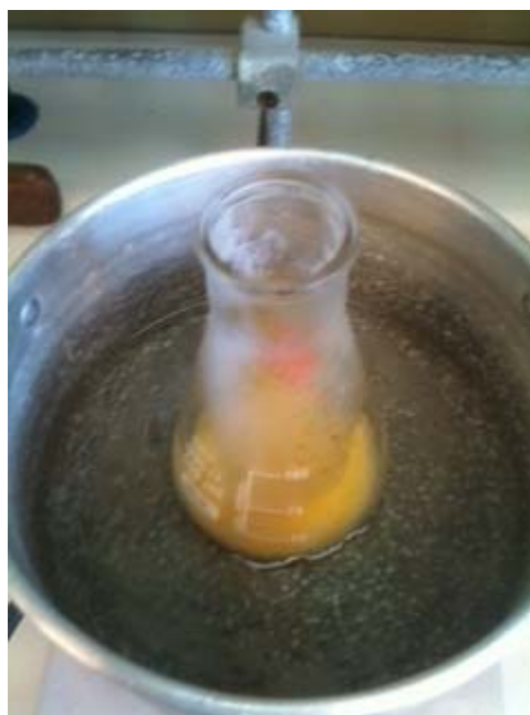
Fig. SM 4.1.1.2.4. Addition of perbromide to stilbene
