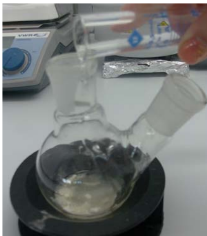
Figure SM 4.1.1.1.1. The cinnamic acid solubilization in \text{CH}_2\text{Cl}_2
